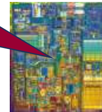
2000 - Intel Pentium 4 42 million transistors 1.5GHz; 224 mm 2
